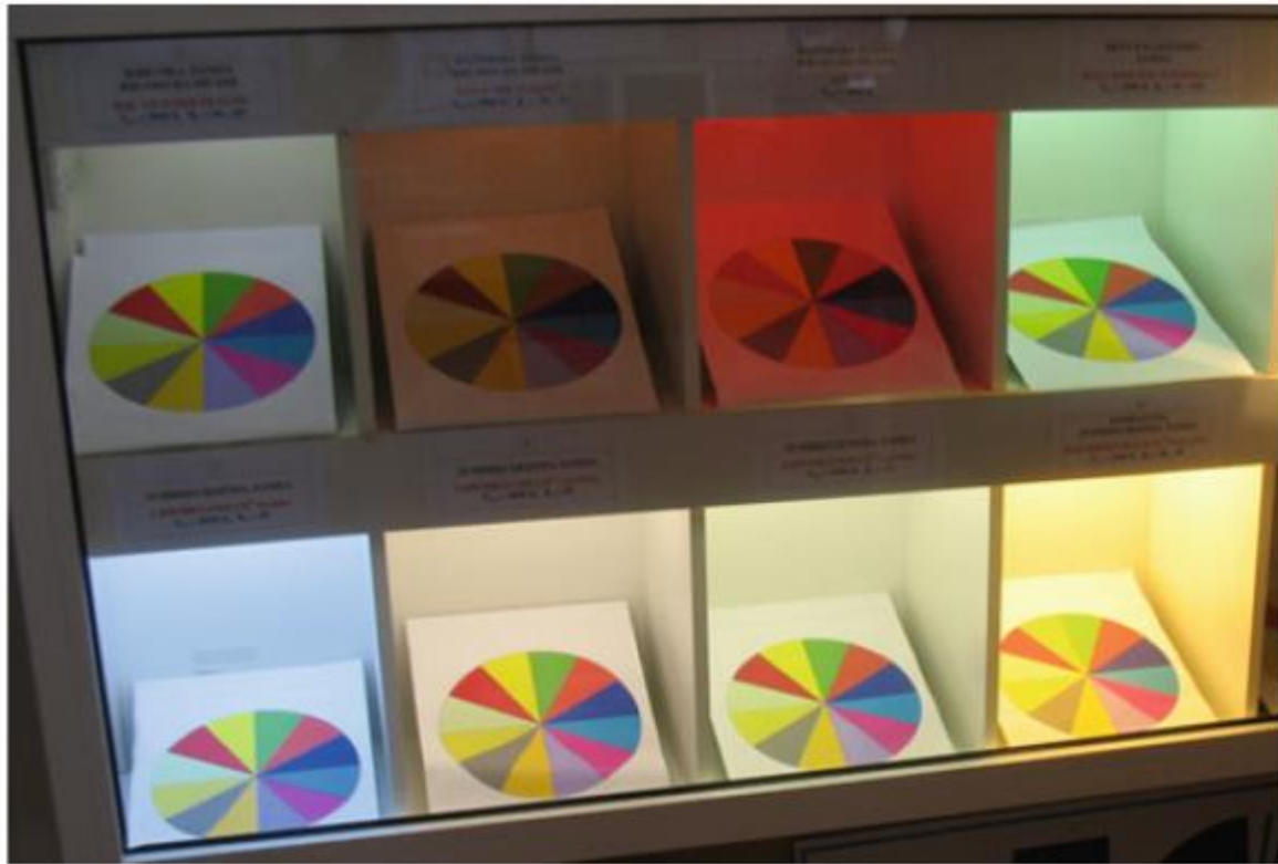
Figure 10 | Visual Comparison of Color Rendering for Different Lamp CRI Values, (Pavlovic, 2020)
