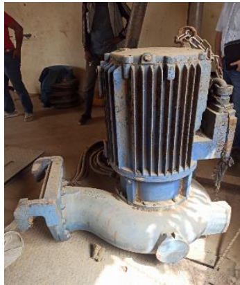
Figure 3 | Low Efficient and Nonoperating Pump, (© IfaS)
