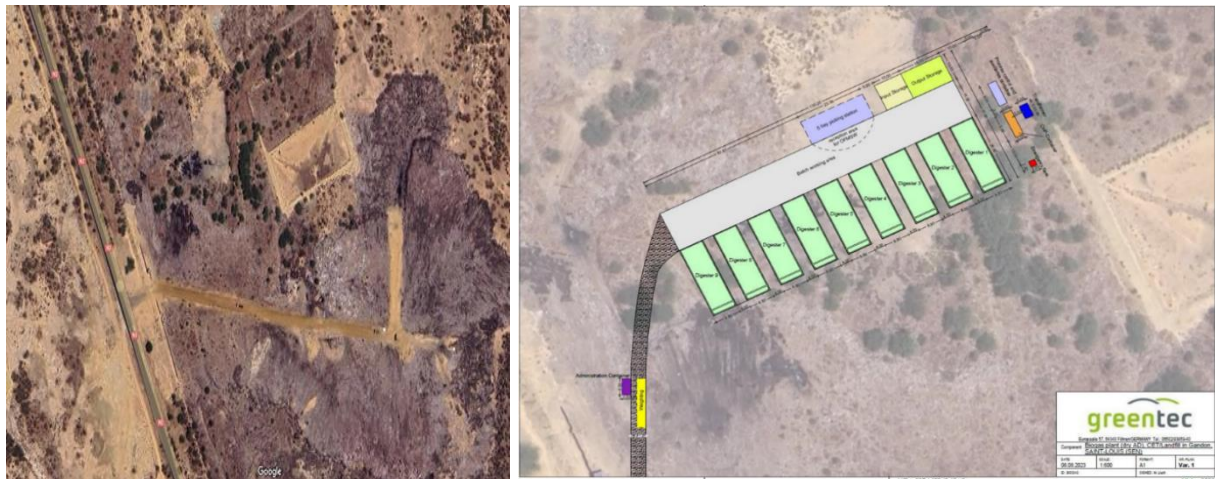
Figure 24 | Aerial View of Gandon Landfill Location and Layout Design of Dry AD Biogas Plant, (© ÖKOBIT GmbH)
