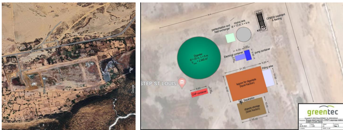
Figure 25 | | Aerial View of STEP Location and Layout Design of Wet AD Biogas Plant, (© ÖKOBIT GmbH)
